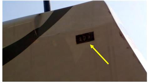
2) The boat's HIN number is engraved on the starboard side near the transom:
