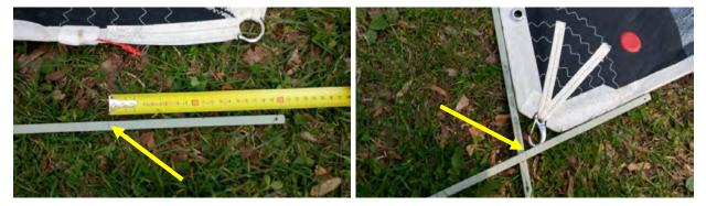
3) Check batten pocket positions relative to ¼, ½ and ¾ leech points, and the outside batten pocket lengths.
