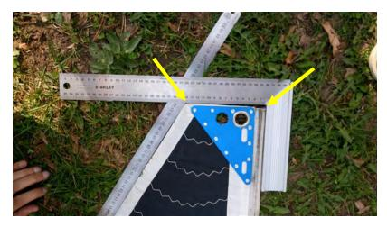
1) Remove battens, flake leech, luff and foot before measuring the respective edge length. Check leech edge shape with a string. Flatten foot before measuring the luff perpendicular.
