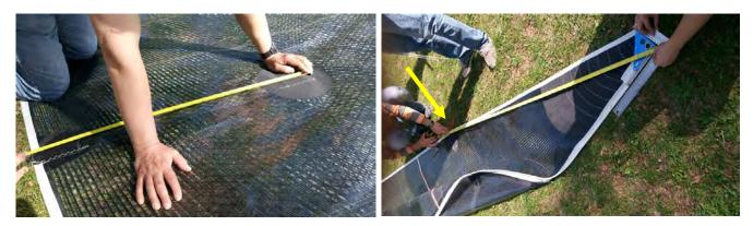
6) Measure the top width with the square and a straight edge to find the aft head point
