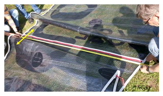
5) Measure the <u>inside</u> batten pocket lengths, and the position of the uppermost pocket from head point. If there is no stitching at the inboard end of the batten pocket, then the inside length is the same as the outside length!
