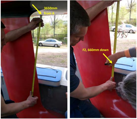
7) Measure the shortest perimeter around the keel at points F1 and F3 with a flat tape:
