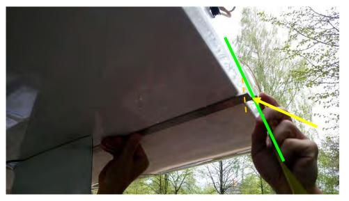
5) Measure the distance between point A and a) the top of the leading edge of the rudder and b) the lowest point of the rudder.
