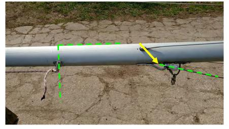
4) Measure the lower and upper points, taper etc. to MDP, and the cross sections with a caliper. Check the tip weight with a small hanging scale or a platform scale. Reverse the weighing position by moving the scale to the lower point and add the two measurements to find the overall mast weight. Make sure that the rigging is not touching the ground or the trestles.
