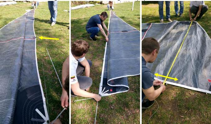
2) The batten tool's specified length for defining the corner points (by extending the sail edges as necessary) is 20cm.
