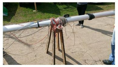
3) Find the rigging point of the forestay. Depending on the attachment type it may be necessary to extend the forestay at the right angle (use the 2610 +/-10mm measurement in F3.2(b) to position the forestay properly) to find where it would intersect the mast spar. Measure the Spinnaker hoist height in the standard way by extending the halyard at 90 degrees to the spar. Mark the taper starting point.
