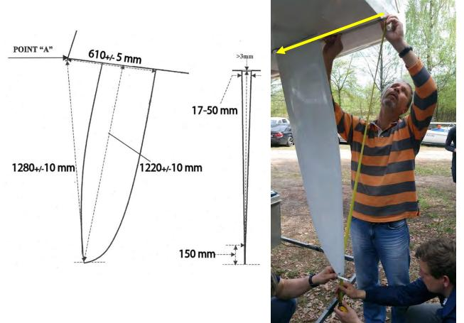
6) Mark the point on the hull centerplane at 3650mm from point A on transom. Measure and mark point F2 and then F1 and F3 on the trailing edge of the keel.
