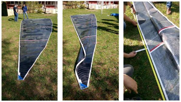
4) Measure the widths at  $\frac{1}{2}$  and  $\frac{3}{4}$  points, adding the hollow if any.
