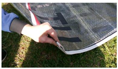
3) Open the sail and flake it along the leech. Measure and record any leech hollows at the measurement points.
