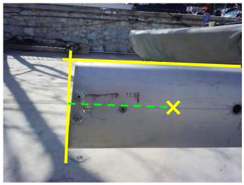
Raise all halyards into sailing position and tie the rigging on the lower point to facilitate weight measurements. Support the mast on two trestles, one at the lower point and one at the upper point.
